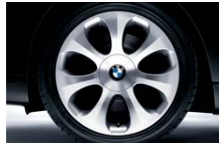
□ 19 x 8.5 front, 19 x 9.0 rear Ellipsoid Spoke (Styling 121) cast alloy wheels and 245/40R-19 front, 275/35R-19 rear performance run-flat tires. 1
