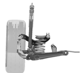
The Multi-link double wishbone rear suspension benefits from increased damper rebound stroke and improved damper mounting locations
