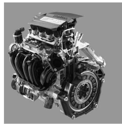
Civic Hybrid 1.3-liter i -VTEC engine and electric motor produce 110 horsepower combined
