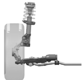
The MacPherson Strut front suspension has a high caster angle and improved toe-control dynamics
