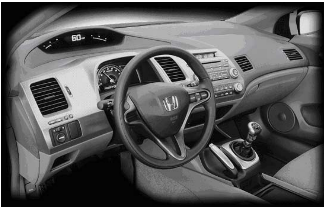
A two-tier instrument panel takes advantage of the generous dashboard space from the steeply angled windshield. This allows for improved positioning of meters and it creates a large sense of space in the vehicle. (Civic Si shown)
