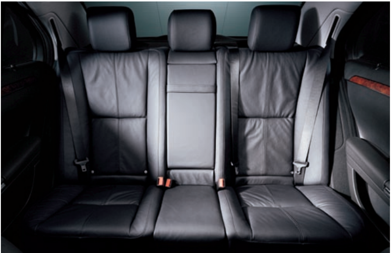
Rear bench seat with electrically adjustable outer seats including PRE-SAFE® positioning function
