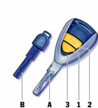
A - Main key 1 - Central locking button 2 - Luggage compartment lid button 3 - Light-emitting diode B - Spare key
