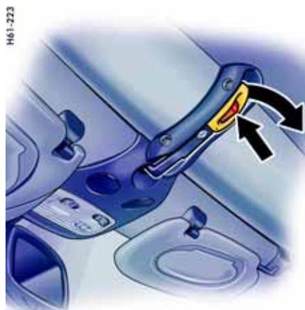
5. Press red lock button of the front locking lever. Fully open locking lever.
