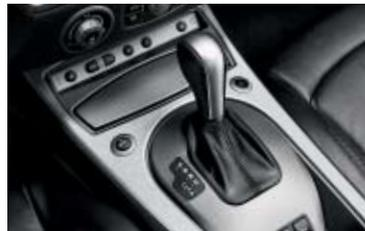
□ **5-speed automatic gearbox with Steptronic**, Adaptive Transmission Management (ATM), Shift-/Interlock; with Steptronic, it is also possible to change gear manually without a clutch.
