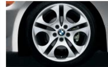
□ Z4 3.0i Sport Package with Ellipsoid (Styling 107) cast-alloy wheels, 18x8.0 front, 18x8.5 rear; and 225/40R-18 front, 255/35R-18 rear run-flat tires.<sup>1</sup>
