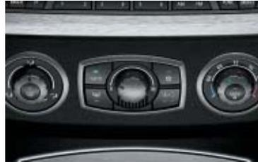
□ **Automatic climate control system** is a new BMW roadster comfort feature. In addition to selecting a specific cabin temperature, occupants can choose from a stepless range of fan speeds, and automatic or manual airflow and recirculation. The automatic recirculation control activates whenever certain air pollutants are detected. The system also includes defrost/demist and Max A/C functions.
