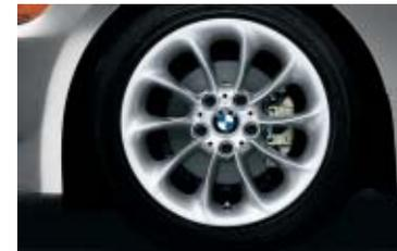
□ Z4 2.5i Sport Package with 17 x 8.0 Turbine (Styling 106) cast-alloy wheels and 225/45R-17 run-flat tires.<sup>1</sup>
