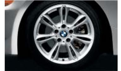
■ Z4 roadster 3.0i with 17 x 8.0 Twin Spoke (Styling 103) cast-alloy wheels and 225/45R-17 run-flat tires.
