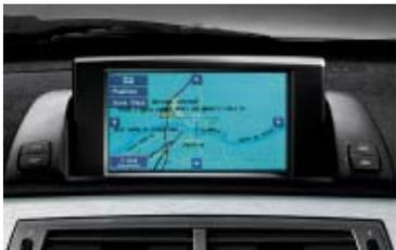
□ **Integrated navigation system**, new in the BMW roadster, covers the entire United States with a single DVD. The pop-up, glare-free monitor is mounted atop the dashboard. When not in use, it retracts back down, out of sight.
