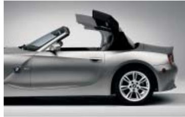
□ **Fully automatic, power softtop** is completely automated. To open or close it, press a button at the front of the center console. The top automatically unlatches from the header and folds down neatly. An interior lining helps reduce wind noise and enhances insulation. Available in Black, Gray and Dark Beige.
