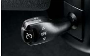
□/■ **Cruise control** lets you store a chosen speed over 18 mph. It can be activated by using a switch located on the left side of the steering column. (opt. or incl. in Z4 2.5i Premium Package; std. in Z4 3.0i)
