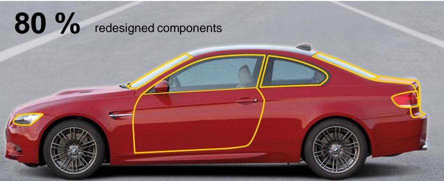
20 % of parts identical with BMW 3 Series Coupe: (rear lights, rear lid, supporting vehicle structure, doors, windows, front lights)
