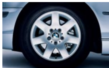
16 x 7.0 Star Spoke (Styling 45) alloy wheels and 205/55R-16 all-season tires work with Dynamic Stability Control to help maximize 325i and all-wheel drive 325xi traction.
